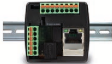
Mounting example in 60 mm switch box or on top-hat rail
